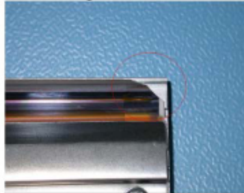
Chipped indication at right print head
